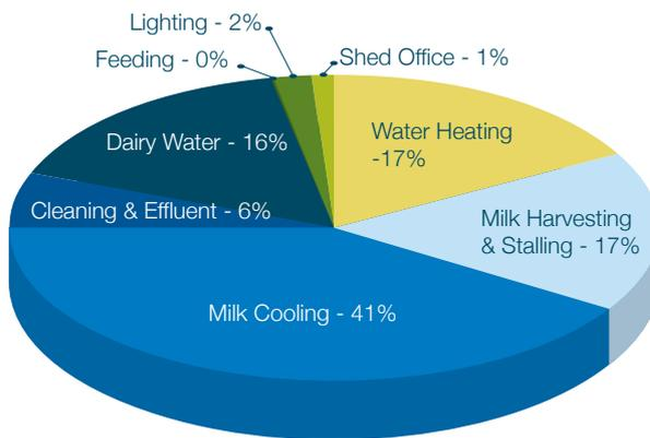
Figure 1: Breakdown of power usage at the dairy meter
